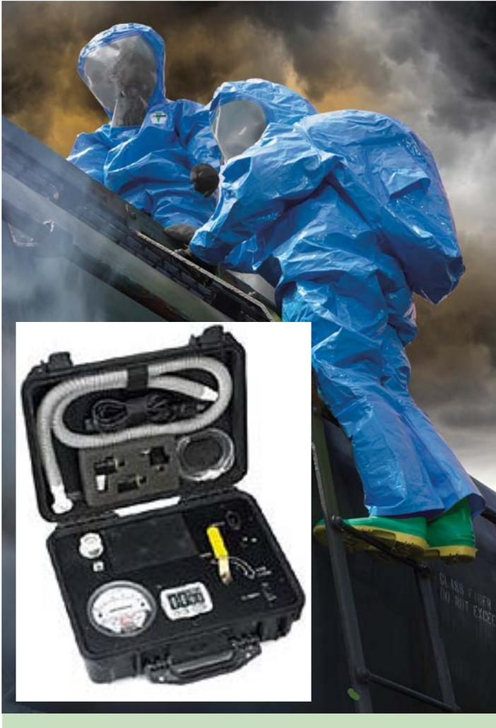
A maintenance program for any EN Type 1 or level A gas-tight suit should include regular internal pressure testing to ensure the suit remains air-tight and leak-proof. This portable pressure test kit includes everything you need to conduct a pressure test on your Interceptor suits
