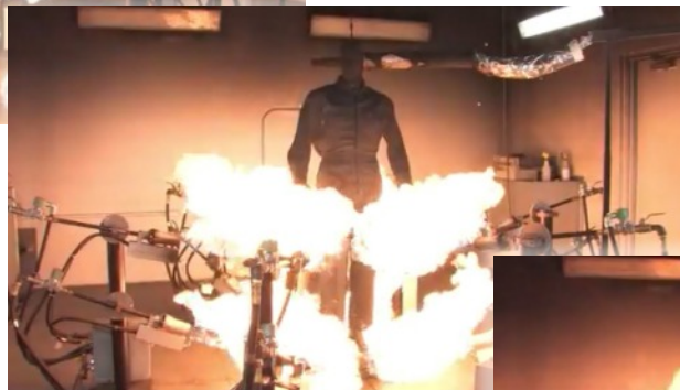
The pictures show three stages in a Thermal Mannequin test - the mannequin wearing an aramid TPG, and the initiation and continuation of the burn
