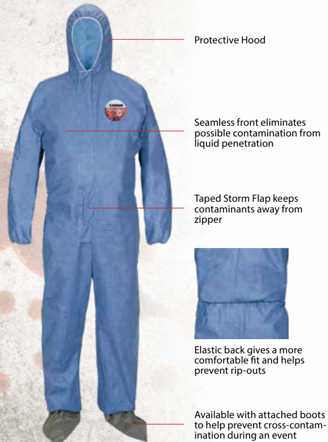
MicroMax ® VP fabric construction creates a protective barrier between the wearer and possible bloodborne pathogen contaminants.
