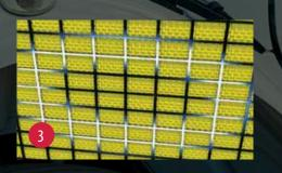
The charge dissipates evenly over the full surface via the carbon grid, leaving a safe lowdensity charge.
