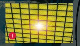
A charged surface comes near or touches the neutral dissipative surface of the fabric.
