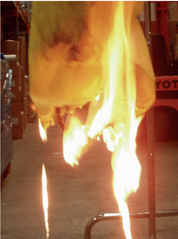
In contact with flame standard disposable fabrics will ignite, burn, drip molten, burning debris and adhere to a TPG worn beneath- actually increasing body burn - often dramatically. 2
