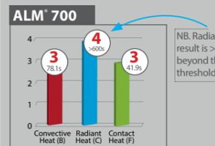
NB. Radiant heat result is >600s - well beyond the Class 4 threshold of 95s.
