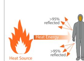
Aluminium has a radiant heat reflective co-efficient of 93-97%.
