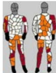
This test produces a body map showing Predicted 2nd and 3rd degree burns and so indicates how effectively a garment protects the wearer.
