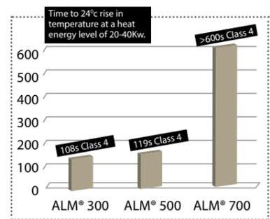
Although all 3 ALM® garments are measured as Class 4. ALM® 700 provides a much higher level of protection - and therefore facilitates greater working times and more protection, than 300/500.
