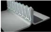
A serged seam joins two pieces of material with a thread that interlocks. This is an economical stitching method for general applications. This stitching method is generally not used for chemical protective clothing. It is more commonly found on disposable clothing where dry particulates are a concern.
