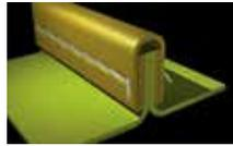
A bound seam joins two pieces of material with an overlay of similar material and is chain stitched through all of the layers for a clean finished edge. This provides increased holdout of liquids and dry particulates.
