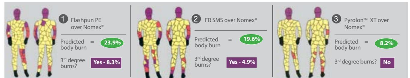
The testing shows that both standard disposables such as Flashpun and FR SMS garments result in higher predicted body burn with very little difference. Only Pyrolon™ garments result in a dramatic reduction in predicted body burn.
